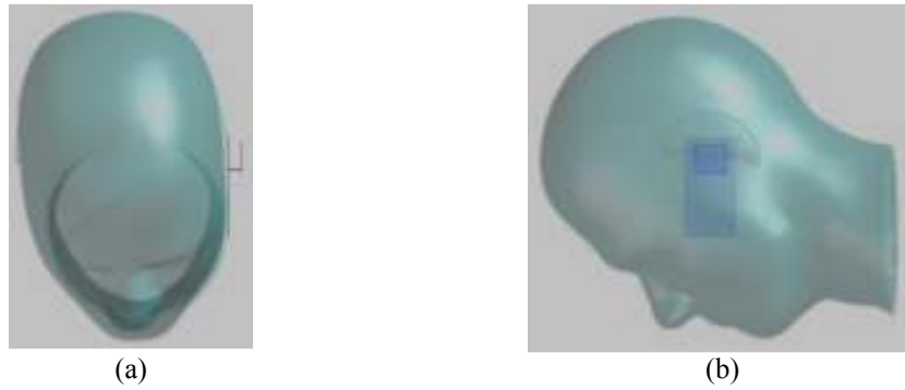
Fig. 2. PIFA and SAM Position (a) Front view (b) Side view
